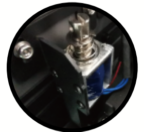
Auto height detector Up to 100 mm thickness substrate
