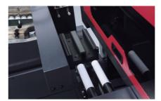
The fixture set supports different size fixtures for tubes with different lengths and diameters. The replacement of the fixture is simple and convenient.
