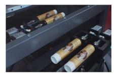
The structure of 2 x 2 operation stations achieves the loading, printing, curing and unloading of two tubes in groups alternatively.
