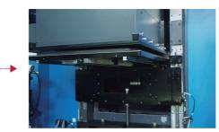
The compact **Print Head Maintenance** Module allows automatic purging, wiping and capping for convenient unattended operation.
