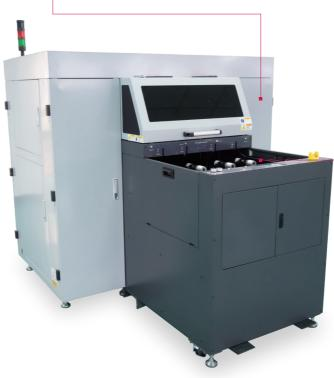
Based on an all-in-one design concept, the small and compact **Print Head Maintenance Module** allows automatic purging, wiping and capping for convenient unattended operation.
