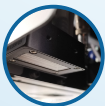
4 water-cooling LED UV lamps
