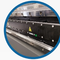
Linear motor, Metal grating & Dual silent linear guides
